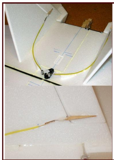
**18.** If incorporating rudders, install the control hardware now. Rudders are not required, but are helpful for improved control at high alpha and for better aerobatics.
