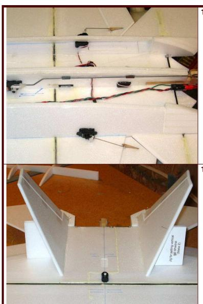
**16.** Next install the flaperons. Cut a 45 degree bevel in the leading edge of the flaperons using a ruler and a hobby knife, and then sand the trailing edges to a tapered shape. Then hinge the flaperons with strips of 3M Satin tape top and bottom. Trim as necessary to provide a small and parallel gap from the leading edge of the stabilators.
