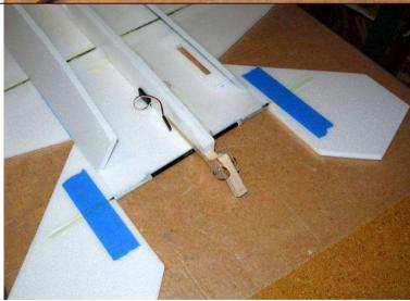
**9.** Sand the leading edge of the stabilators to a well-rounded shape, and the trailing to a tapered shape. Apply a strip of 3M Satin tape to the leading edge for smoothness and durability.
