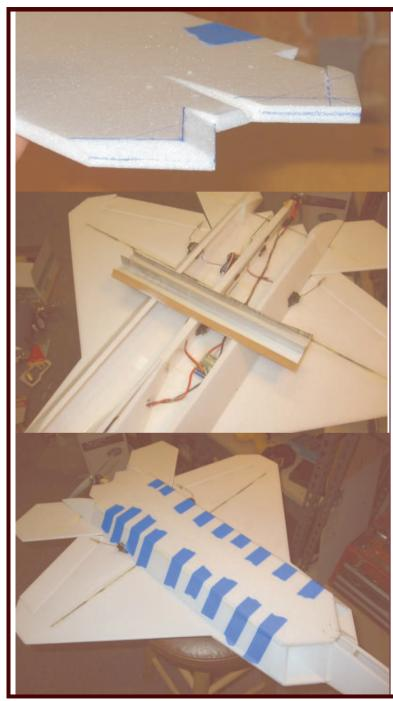
23. Next make and install the aft fuselage bottom piece. Begin by cutting the bevels in the sides as shown on the plans. Also cut bevels in the exhaust nozzles as shown in the top photo at left. You'll also need to carve a small notch in the center between the exhaust nozzles to provide clearance for the thrust vectoring pushrod and clevis (test fit the part to determine how much clearance is required).
