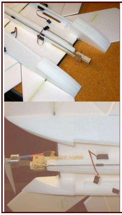
15. Laminate the tail boom pieces together using 3M 77 adhesive. Then glue the tail boom blocks to the aft fuselage with epoxy. Note that you'll need to carve out a small channel in the top of the tail boom blocks first to clear the aluminum stabilator pivot tubes. Make sure the tail boom blocks fit tight against the stab pivot tubes, since they provide significant extra strength to the stabilator pivots.
