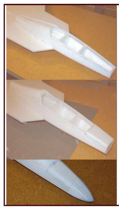
**13.** Glue bulkheads F4 and F5 to the top of the wing in the locations shown on the plans. Then glue the aft part of the upper forward fuselage sides to the top of the wing and the bulkheads. Note how the fuselage sides curve inward as they run aft—you can heat form the foam slightly to attain this curvature. Pins can be used to hold the foam in place as the glue cures.
