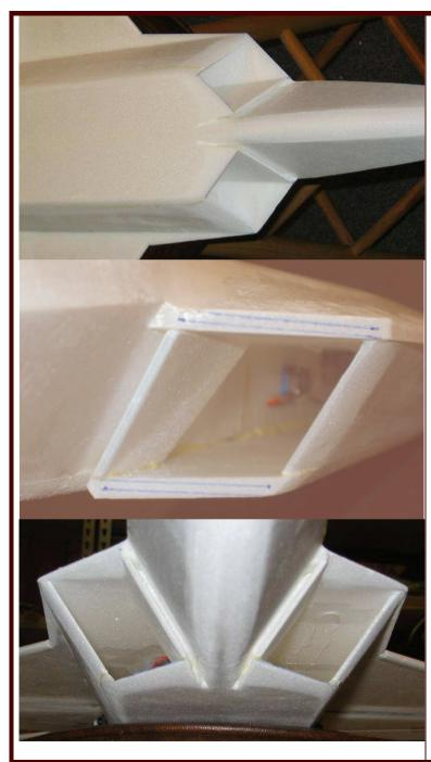
**24.** Now shape the inlets and aft fuselage. Begin by cutting slots in the aft fuselage bottom piece to provide exits for the inlet diverters (see top photo at left). Use a hobby knife inserted between the diverter pieces to cut the slot, and then trim with sandpaper.
