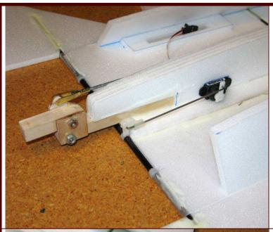
**10.** Install the stabilator servo into the pre-cut slot in the fuselage centerline support (thick CA can be used to hold the servo in place). Make and install a music wire pushrod to the stab control horn. Once everything is properly aligned, glue the stab control horn into place using thin CA.
