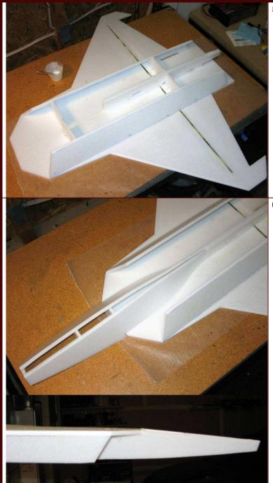
**5.** Laminate the two fuselage centerline support pieces together (3M 77 spray adhesive recommended). Then cut bevels on the edges of the aft fuselage sides as indicated on the plans.
