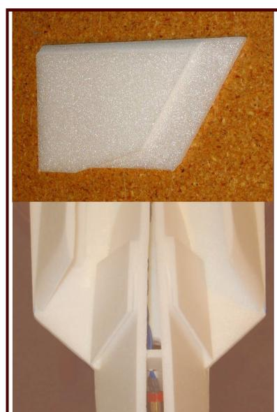
**22.** Laminate the inlet diverter piece and inlet side piece together as shown in the top photo at left, using 3M 77 adhesive. Make two assemblies. Then glue the assemblies at the front of the inlets as shown in the bottom photo.
