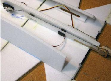
11. Next install the thrust vectoring servo and pushrod. A strong (40+ oz/in torque) metal-geared servo is required since a plastic-geared servo could get stripped if the prop hits the ground during landings. The prototype used a Hitec HS-85MG servo, which worked very well. Install the servo in the precut slot in the fuselage centerline support, securing it with CA.
