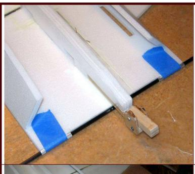
**8.** Glue the completed motor mount into the slot in the aft fuselage centerline support, aligning it to a zero-zero thrust line (no left/right or up/down thrust angle). Use 5 minute epoxy.
