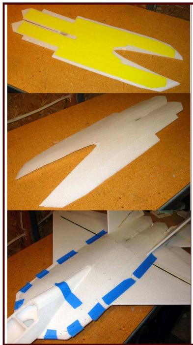
**20.** Next shape and install the aft fuselage top piece. This is perhaps the most challenging aspect of building this model, so take your time. There are many ways to form the curvature required, but I'll describe the particular method I used.
