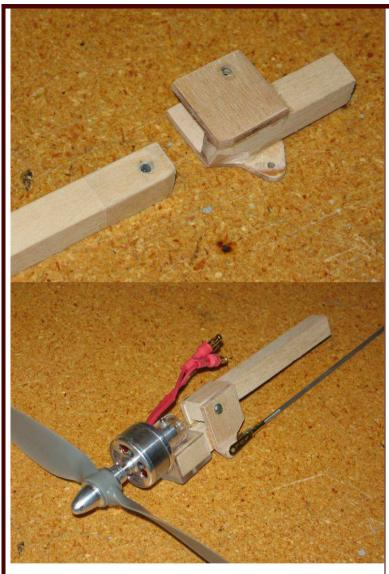
7. Next assemble the thrust vectoring motor mount. This step is optional—you may choose to install a straight motor stick if you don't want thrust vectoring.
