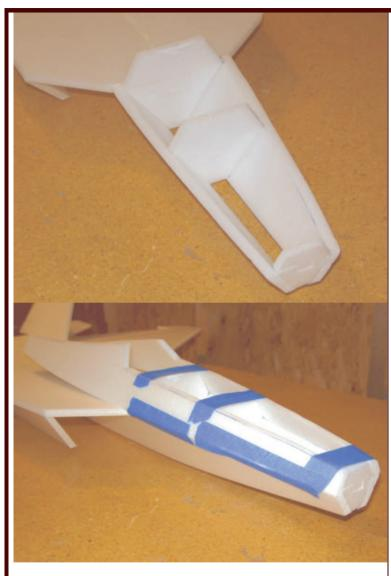
**12.** Use a sanding block to lightly sand the top of the lower forward fuselage until it is flat and even. Then glue on the upper half of each of the three forward fuselage bulkheads.
