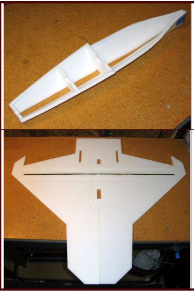
3. Glue the bottom half of the three fuselage bulkheads (the ones with the notch on top) to one of the lower forward fuselage sides at the locations shown on the plans, making sure they are perpendicular. Then set the fuselage sides upright and flat on the workbench, apply glue to the edges of the bulkheads, and then glue the two fuselage sides together.
