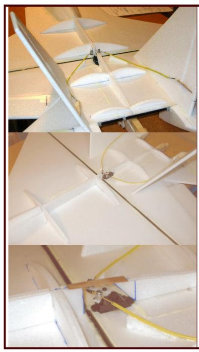
**19.** Glue the turtledeck top spine into place on the wing centerline. Then glue the five turtledeck bulkheads (T1 through T5) into place in the locations shown on the plans.
